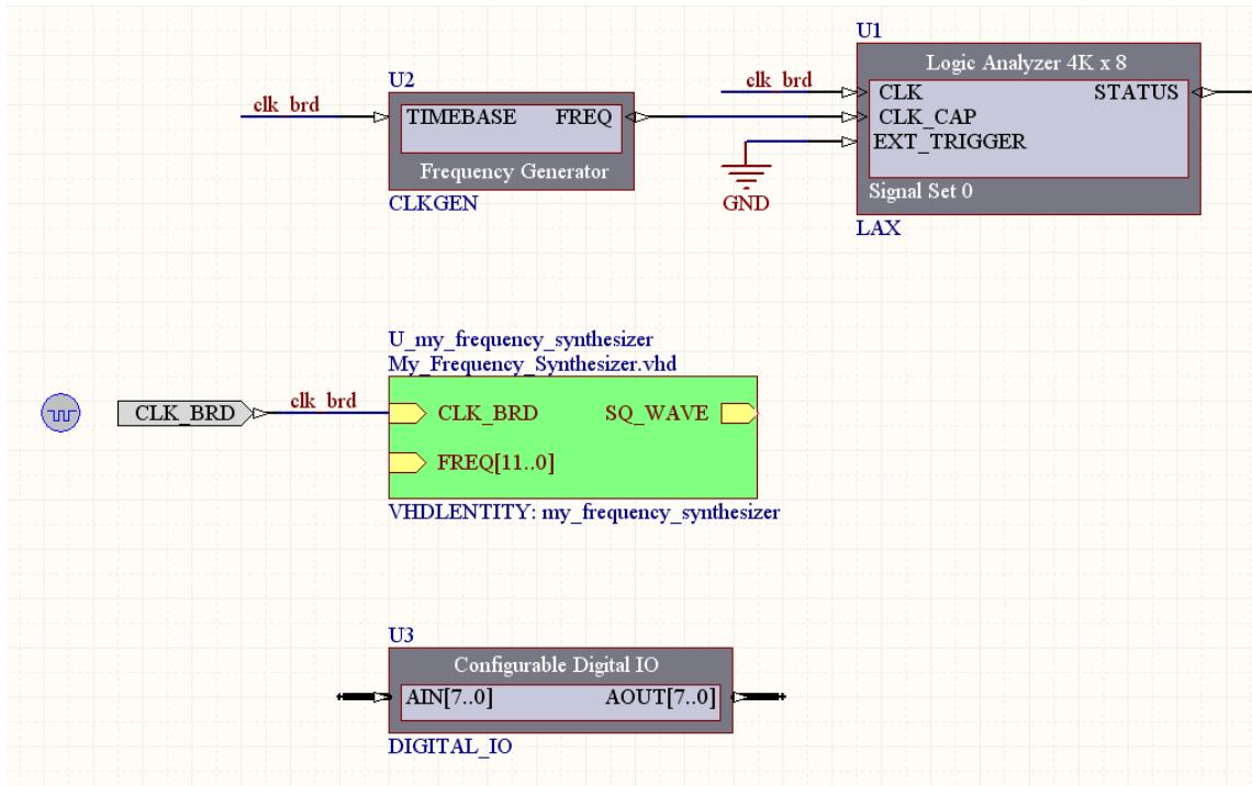
2. Next configure the logic analyzer to receive one input signal by double-clicking on the component symbol and then clicking on the “Configure...” button to bring up the dialog window shown below. Click on the “Add Signal” button and type in the name of the square wave output signal “SQ\_WAVE”. Next set the number of samples to capture to 4K using the drop down box.
