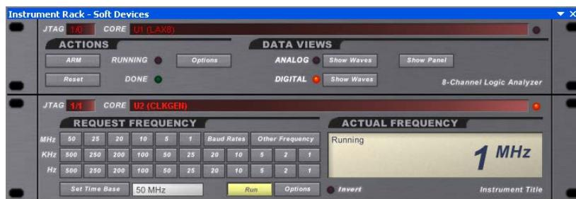
8. Change the frequency generated by the CLKGEN to 20 kHz. Open the “options” dialogue window for the Logic Analyzer and set the clock capture frequency to 20 kHz as shown below.
